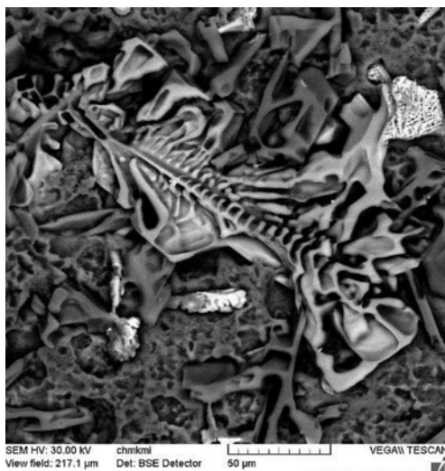
FIG. 5. Morphology of Fe-rich intermetallic phases in as-cast structure of \text{AlSi9Cu3} cast alloy, SEM.
