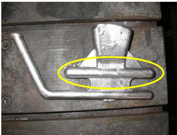
FIG. 1. Metallic mould and molten semi-product: a) metallic mould with semi-product, b) detail of semi-product.
