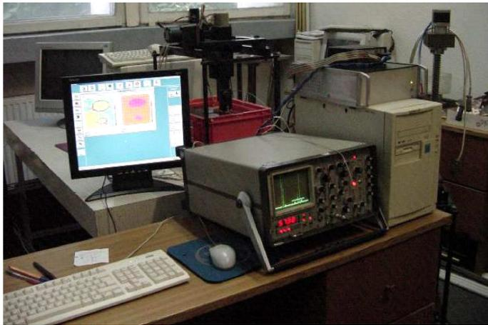
FIG. 5. The experimental set-up for ultrasonic imaging.
