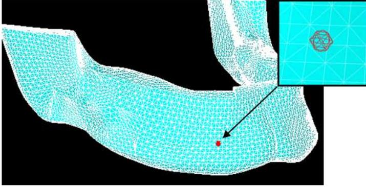
FIG. 1. Finite element model of the mandible with the cyst.
