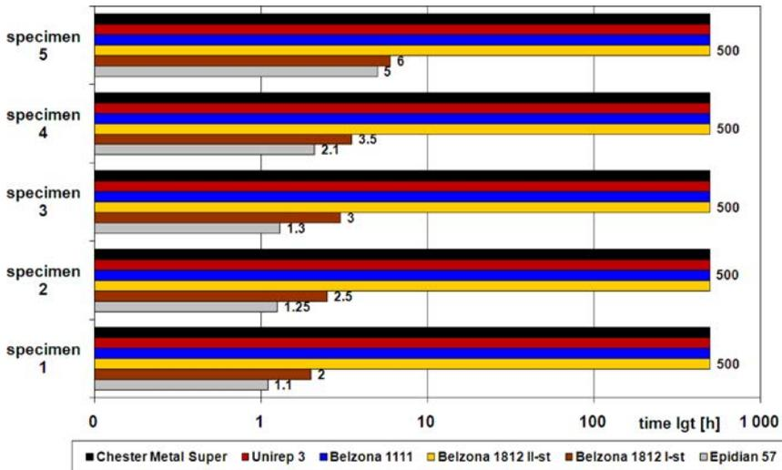
FIG. 8. Static long-term strength of lap joints made of adhesive composites (loaded with a power of 60%  $F_n$  and at a temperature of 60°C).
