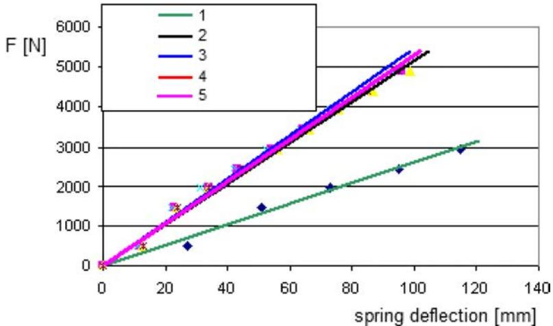
FIG. 5. Characteristics of the springs used in devices with the imposed loads.
