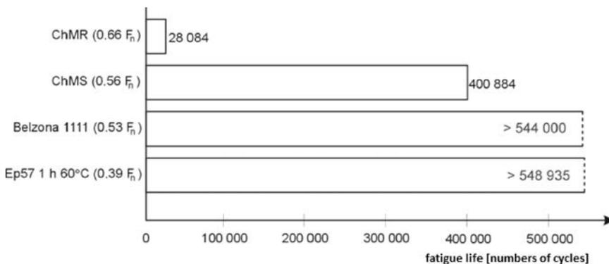
FIG. 14. Comparison of the absolute shear fatigue life of adhesive composites (the maximum load of a fatigue cycle was 1.3 kN for all adhesives).
