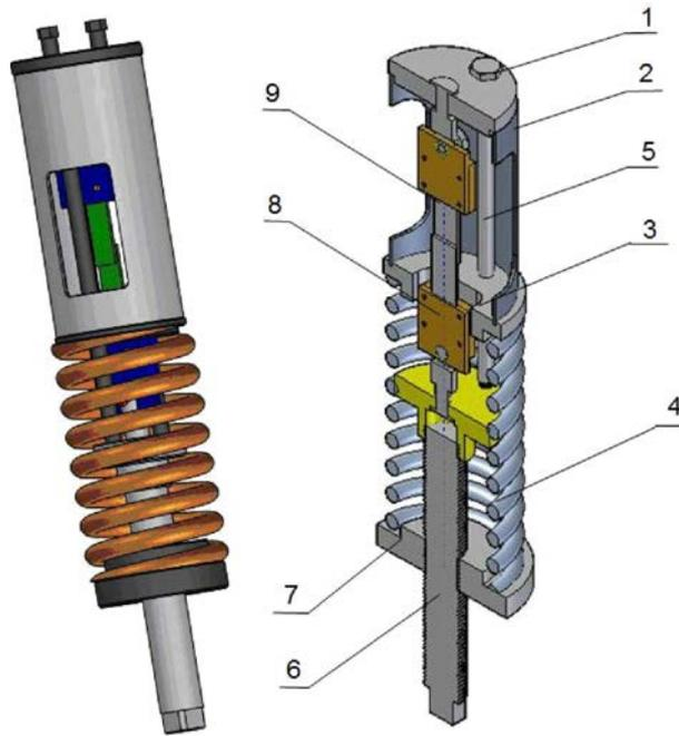
FIG. 3. The device used to determine static long-term strength of adhesive joints: 1, 3 – covers; 2 – spacing sleeve; 4 – spring; 5 – lock screws; 6 – screw tightening the spring; 7 – resistance sleeve; 8, 10 – grips for specimen mounting; 9 – tested specimen [13].
