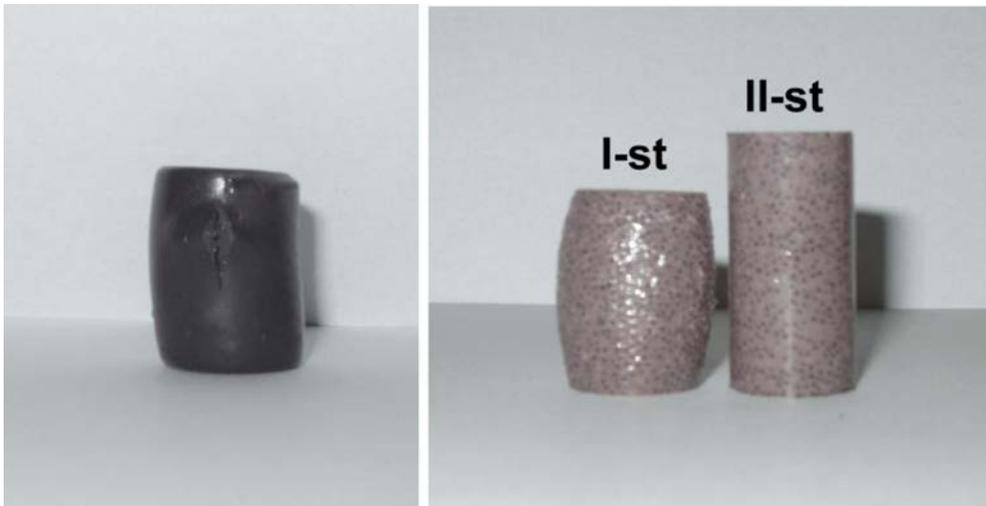
FIG. 6. Unirep 1 and Belzona 1812 (after single-stage stage curing) adhesive composites after a few minutes from the moment of 30 MPa load at a temperature of 60°C.
