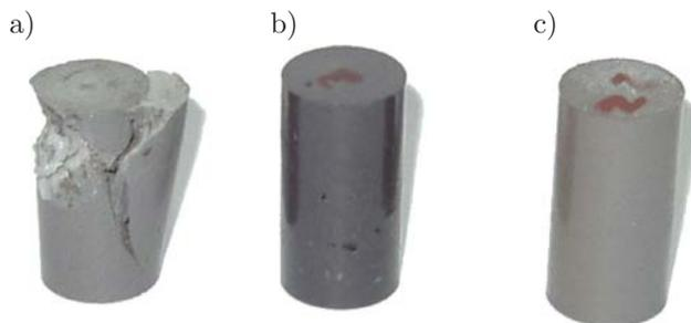
FIG. 11. View of specimens after fatigue tests: a) Chester Metal Super, b) Unirep 3, c) Belzona 1111.
