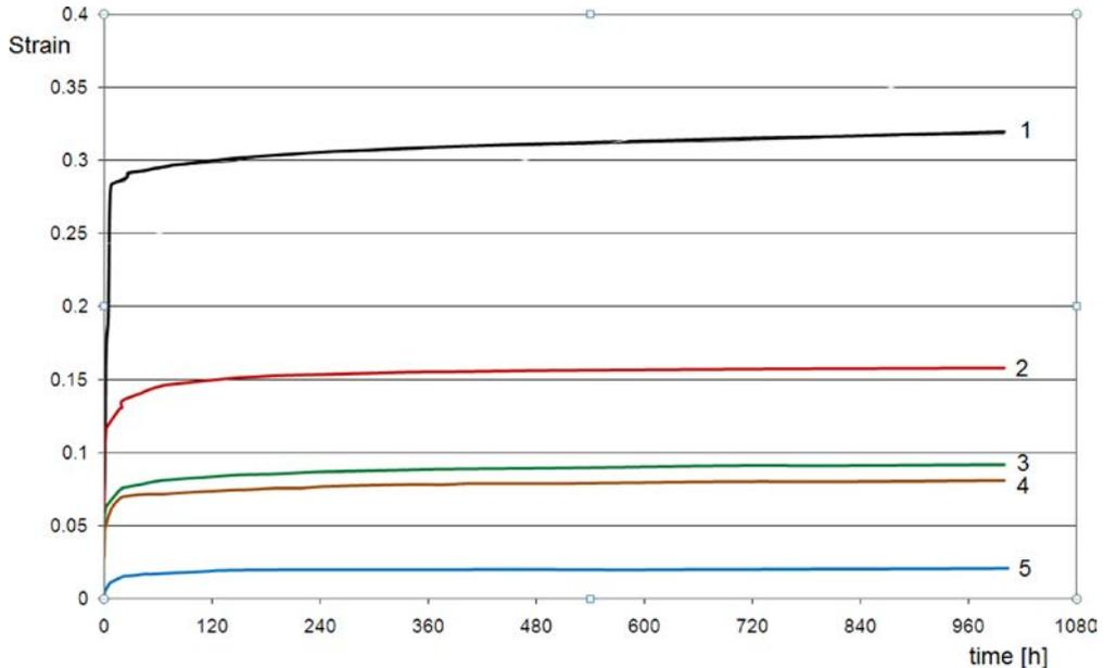
FIG. 7. Creep curves of the adhesive composites in the temperature of  $60^{\circ}\text{C}$  with load causing normal stresses of 30 MPa in the examined specimens (1 – Epidian 57, 2 – Chester Metal Super, 3 – Belzona 1111, 4 – Unirep 3, 5 – Belzona 1812 – II st.).
