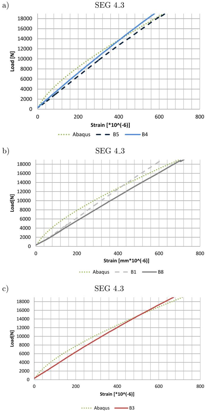
FIG. 4. The force – strain relation obtained from the numerical model and SEG 4.3 readout for the beams: a) reinforced at the tensioned flange, b) reinforced at the compressed flange, c) bare beams.
