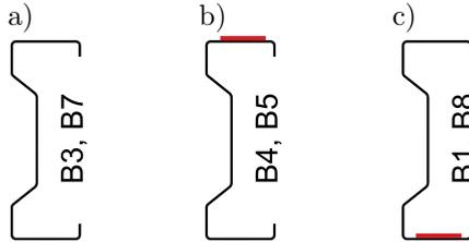
FIG. 1. Layout of CFRP tapes on the examined thin-walled beams: a) bare beams, b) CFRP tape bonded to the tensioned flange, c) CFRP tape bonded to the compressed flange.
