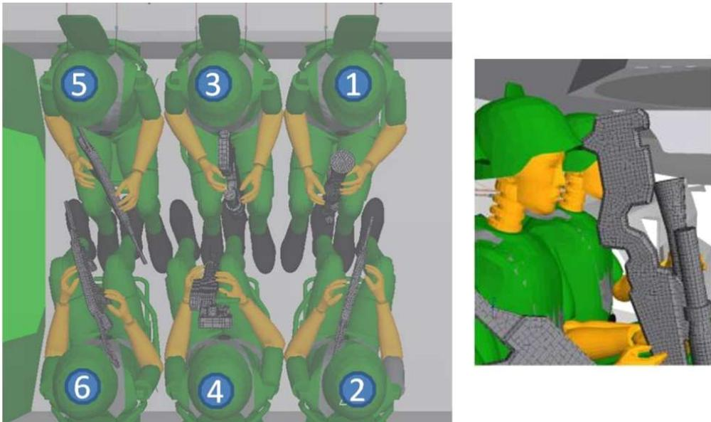
FIG. 3. Deployment of soldiers in the vehicle – left, moment of weapon hitting soldier's helmet – right.
