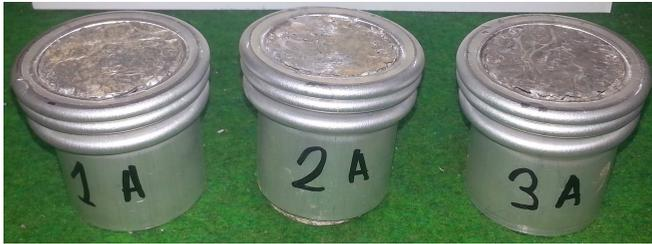
FIG. 11. Samples of circular aluminium profile filled with low density aluminium foam, after the dynamic compression.
