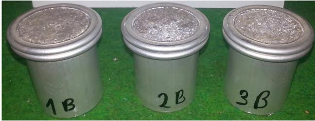
FIG. 13. Samples of circular aluminium profile filled with high density aluminium foam, after the dynamic compression.
