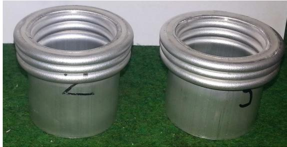
FIG. 7. Samples of circular aluminium profile without filling, after the dynamic compression.
