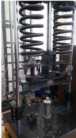
FIG. 4. Spring hammer testing apparatus used the for dynamic impact tests.
