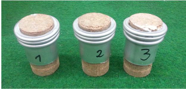
FIG. 9. Samples of circular aluminium profile filled with Cork\_NL25, after the dynamic compression.
