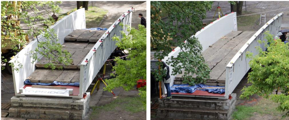
FIG. 2. Footbridge loaded during tests U1 (left side) and U3 (right side).
