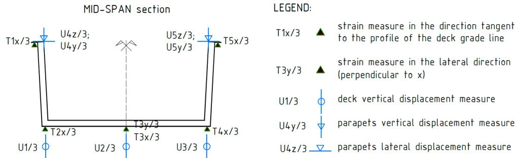
FIG. 3. Location of measurement points in mid-span section of the footbridge.
