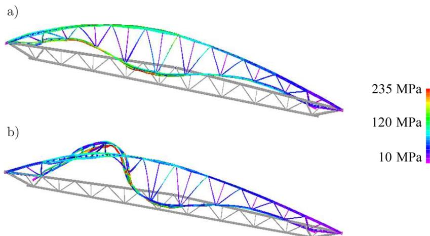
FIG. 6. Deformation at the limit state (GMNIA) for the truss with braces of stiffness:
