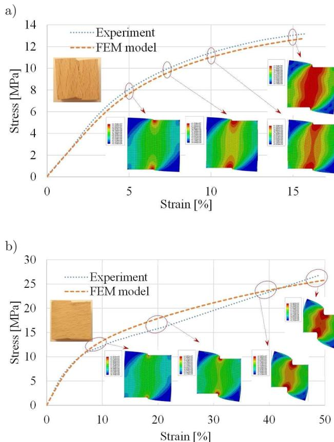
FIG. 7. a) The stress-strain curves for beech specimen sheared in radial direction at 20°C and 18% moisture, b) the stress-strain curves for beech specimen sheared in longitudinal direction at 20°C and 18% moisture.
