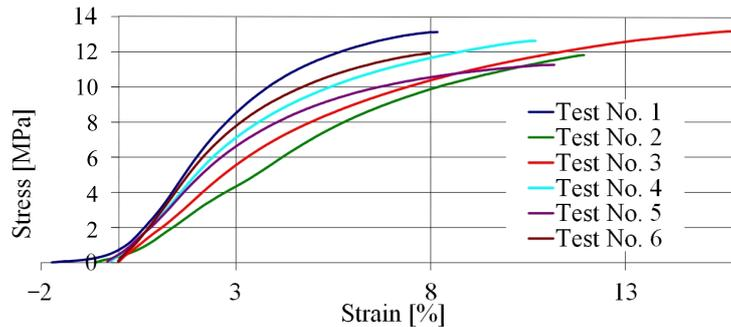
FIG. 5. The stress-strain curves for six beech specimens sheared in radial direction at 20°C and 18% moisture content.
