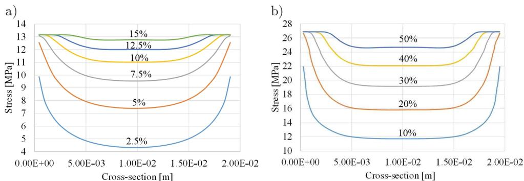
FIG. 8. a) The stress-cross-section distance curves for beech specimen sheared in radial direction, b) the stress-cross-section distance curves for beech specimen sheared in longitudinal direction.
