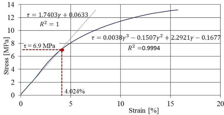
FIG. 4. The stress-strain curve for beech specimen sheared in radial direction at 20°C and 18% moisture.
