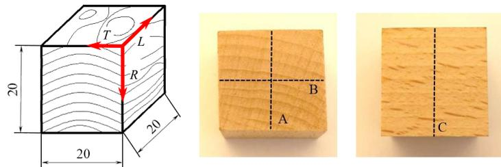
FIG. 2. a) Dimensions of specimen, b) edges of shearing: A – radial direction, B – tangential direction, C – longitudinal direction.
