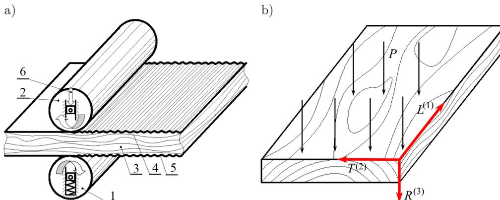
FIG. 1. a) Treatment of the surface layer of natural material by hot rolling: 1 – bottom roller, 2 – top roller, 3 – chipboard, 4, 5 – top and bottom layers of natural veneer, 6 – applied force, b) orientation of wood fibres (anisotropy):  $P$  – load,  $L$  – longitudinal direction, parallel to fibres, and two directions perpendicular to fibres:  $R$  – radial and  $T$  – tangent.
