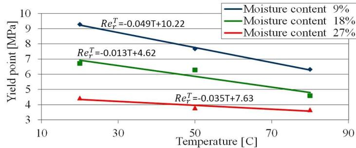
**FIG. 6.** Yield point vs. temperature for three moisture content levels – beech, radial direction.
