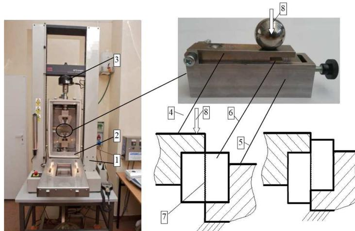
FIG. 3. MTS strength tester including climate chamber: 1 – strength tester, 2 – climate chamber, 3 – load cell (measuring the applied force), 4 – movable jaw of shear test device, 5 – fixed jaw of shear test device, 6 – specimen, 7 – surface of cutting, 8 – load of strength tester.
