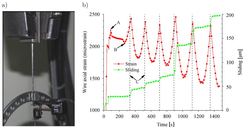
FIG. 1. a) The experimental set-up of the preliminary protocol, b) axial strain and slippage vs. time [2].
