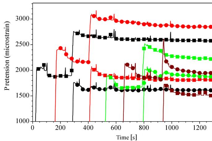
FIG. 3. Time variation of the pretension during the assembling stage.
