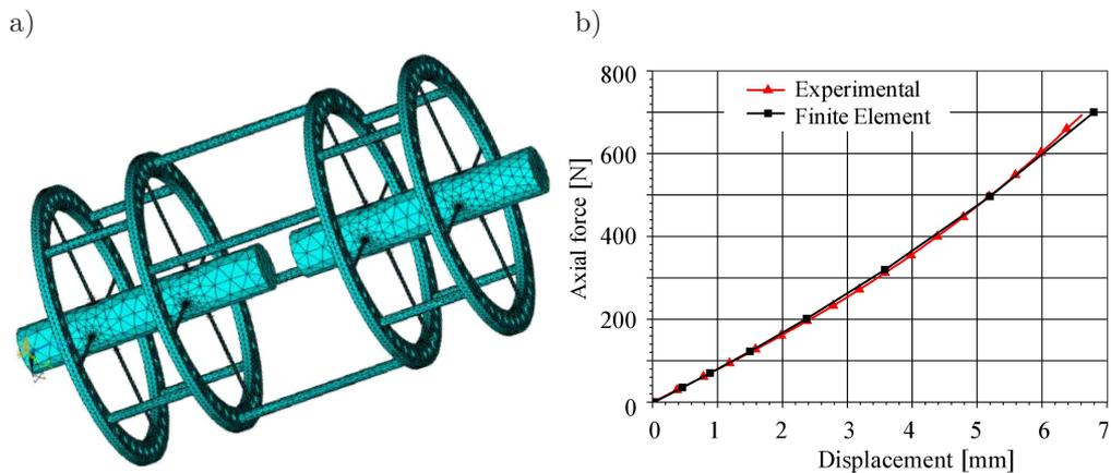
FIG. 5. The finite element model (a) and its validation according to the experimental data (b).
