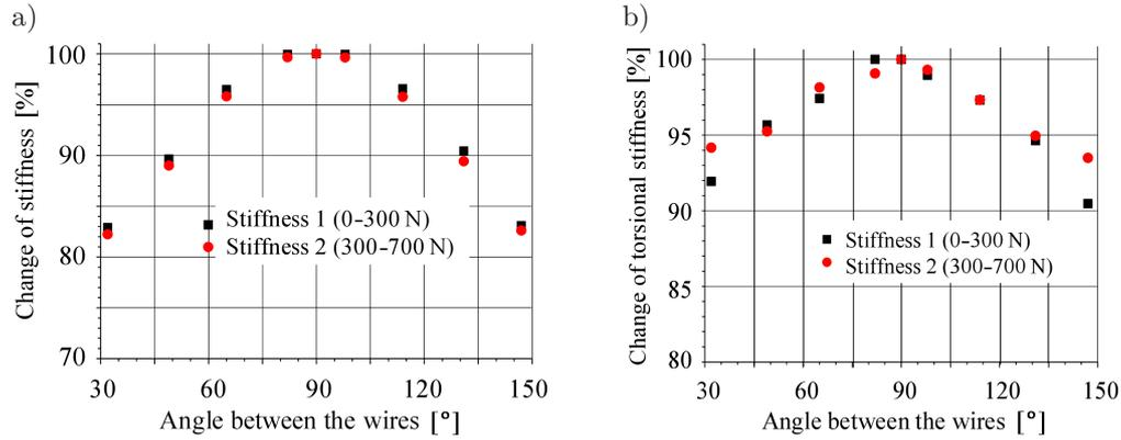
FIG. 6. The influence of the wires' angle on the fixator's axial- (a) and torsional-stiffness (b).
