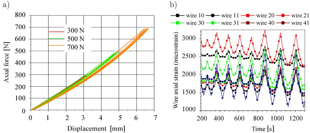
FIG. 4. The axial force versus the displacement of the “bone” (a) and the time variation of the pretension of all wires during the loading-unloading loops (b).
