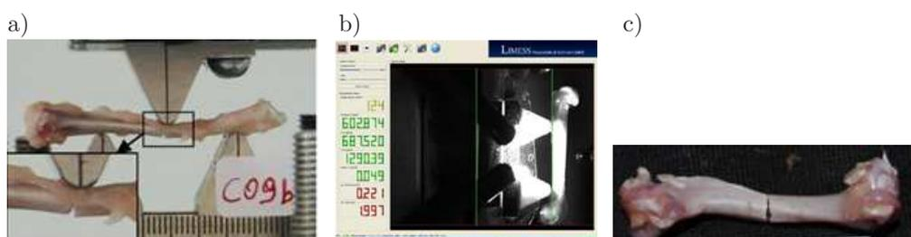
FIG. 1. Typical specimens: a) while loaded (at the onset of fracturing), b) as it is seen through the screen of the video extensometer before the onset of the loading procedure and c) after the test.
