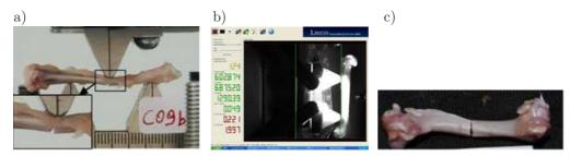
FIG. 1. Typical specimens: a) while loaded (at the onset of fracturing), b) as it is seen through the screen of the video extensioneter before the onset of the loading procedure and c) after the test.
