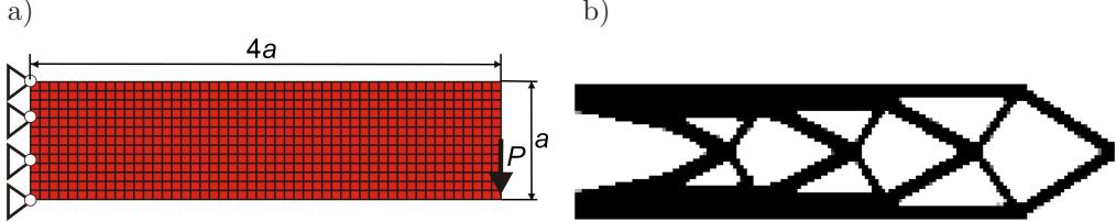
FIG. 4. a) Initial structure, and b) final topology.
