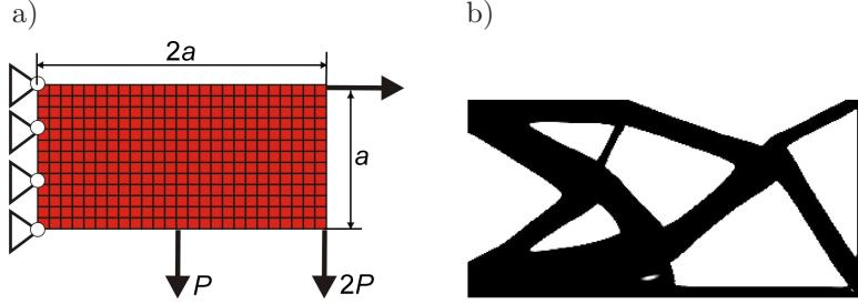
FIG. 3. a) Initial structure, b) and final topology.
