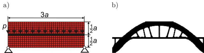
FIG. 6. a) Initial structure, and b) final topology.
