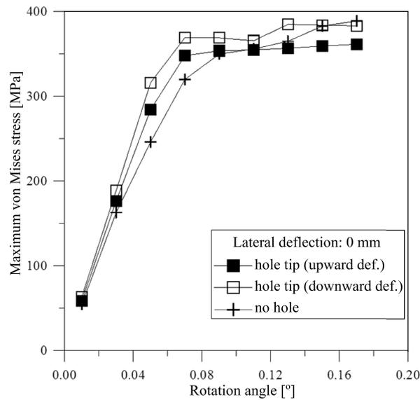
FIG. 6.  $\sigma_{V\_max}$  versus RA at 0 mm deflection.
