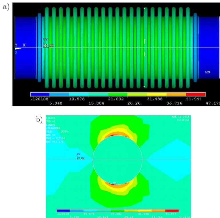
FIG. 2. a)  $\sigma_V$  by axial movement ( $\sigma_{V\_max} = 18$  MPa),
