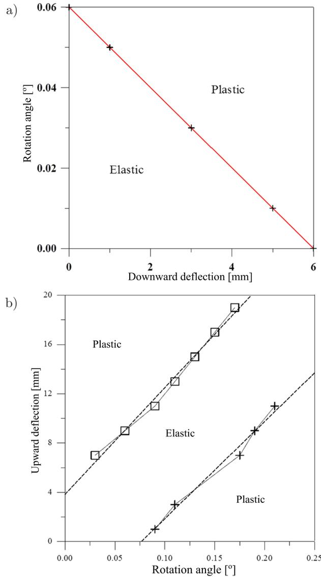
FIG. 7. a) Elastic-plastic boundary with DD and RA, b) elastic-plastic boundary with UD and RA.
