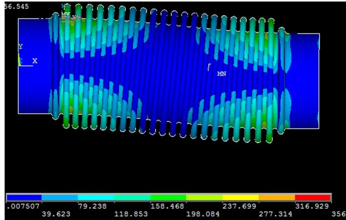
FIG. 3.  $\sigma_V$  by  $0^\circ$  RA and 7 mm DD.
