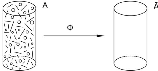
FIG. 1. Damaged and fictitious undamaged configurations.
