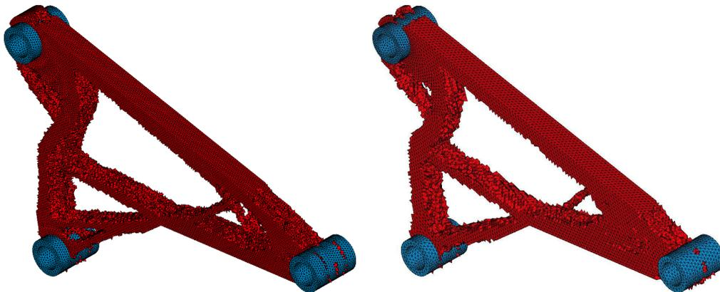
FIG. 2. Final topology for regular (left) and irregular (right) lattice.
