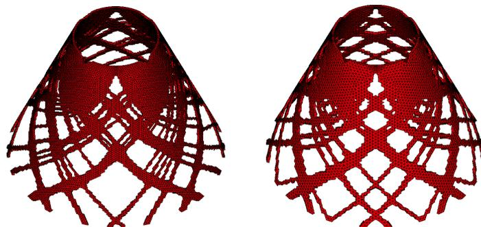
FIG. 4. Final topology for regular (left) and irregular (right) lattice.
