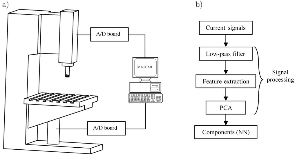
FIG. 1. a) Schematic diagram of the experimental set-up, b) schematic diagram of the monitoring strategy.
