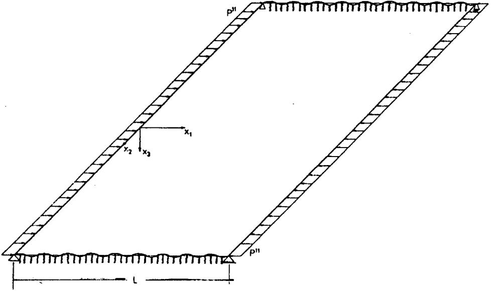
FIG. 2. A scheme of a long rectangular plate compressed along the edges in direction of  $x^1$ .
