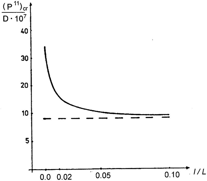
FIG. 3. The smallest value of a critical forces  $(P^{11})_{cr}$  for a long rectangular plate resting on the Winkler elastic foundation versus ratio  $l/L$ , for a microstructural and a orthotropic models.
