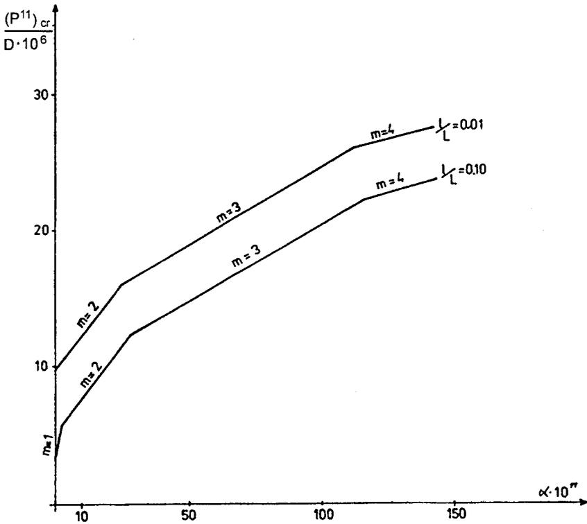
FIG. 4. The smallest value of a critical forces  $(P^{11})_{cr}$  versus parameter  $\alpha$  of the modulus of foundation; the number of half-waves  $m$  and ratio  $l/L$  are used as parameters. Here it assumed that  $k = \alpha \frac{D}{\delta^2}$ .
