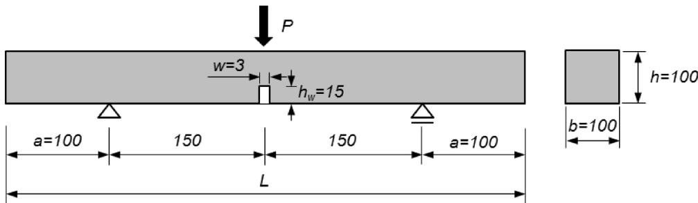
FIG. 3. Geometry and load condition of tested beam.
