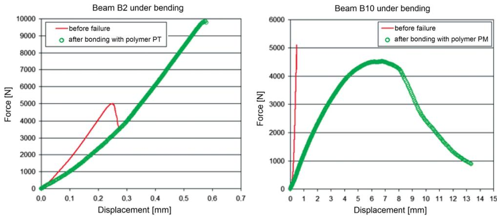
FIG. 5. Force-displacement relation of B2 and B10 beams before failure and after bonding with polymers PT and PM [7].
