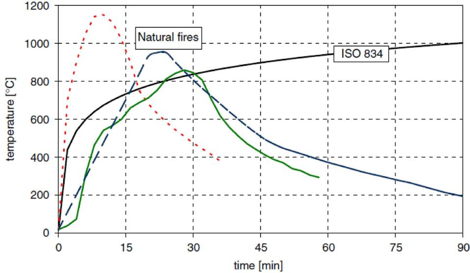
FIG. 1. A comparison between natural fire curves and the ISO 834 curve [8].
