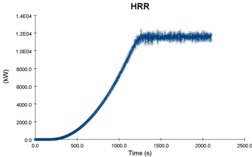
FIG. 12. The evolution of the rate of heat release obtained in the fire dynamics simulator.
