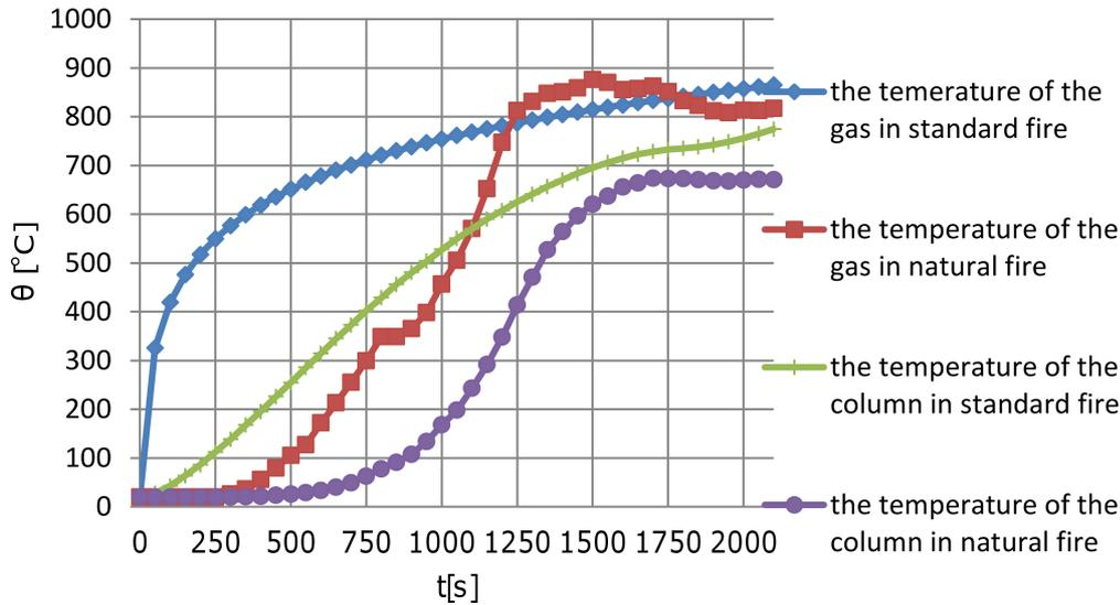
FIG. 13. The rise of the temperature of the unprotected steel column subjected to the standard fire curve ISO 834 and to the natural office fire model.
