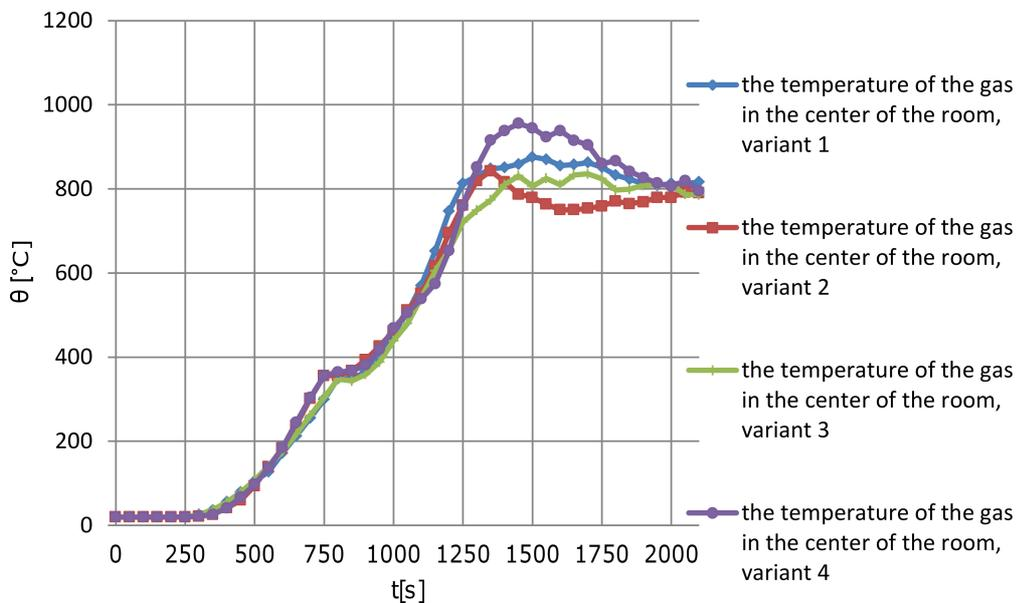
FIG. 7. The temperatures of the gas in the center of the room in all variants.
