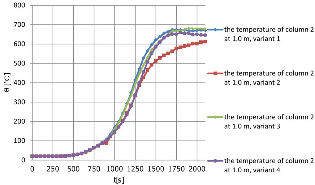
FIG. 10. The temperatures of column 2 at 1.0 m above the ground in all variants.
