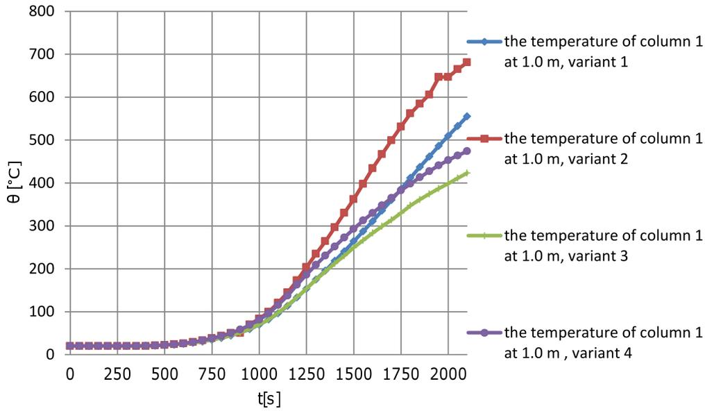
FIG. 8. The temperatures of column 1 at 1.0 m above the ground.
