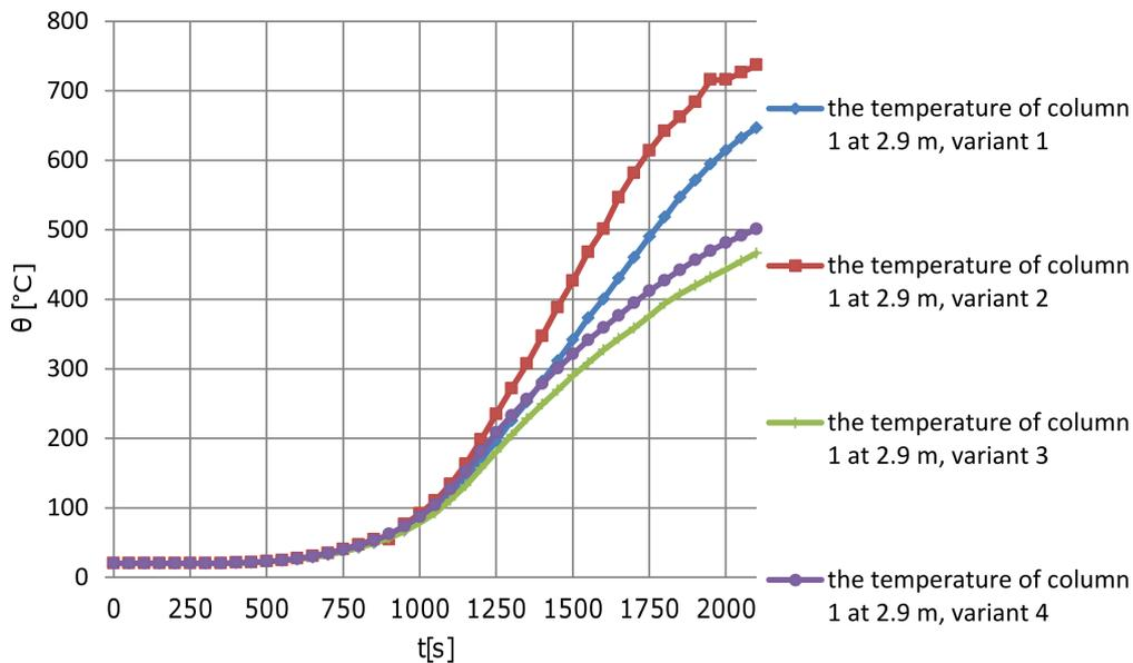
FIG. 9. The temperatures of column 1 at 2.9 m above the ground in all variants.
