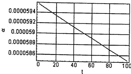
FIG. 7. The sensitivity of the probability of failure calculated for the ultimate limit state due to the time of observation.
