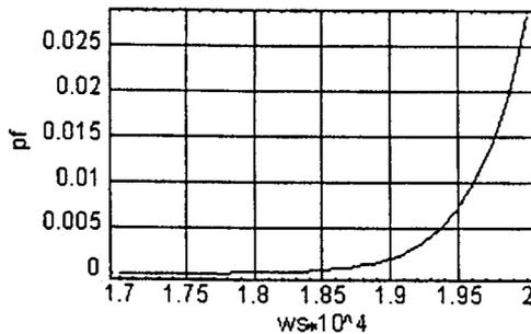
FIG. 4. The probability of failure calculated for the serviceability limit state vs. the expected value of the displacement.
