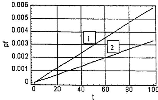
FIG. 3. The probability of failure vs. the time of observation (years), the curve "1" is calculated for the ultimate limit state, the curve "2" for the serviceability limit state.
