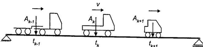
FIG. 2. A model of a bridge beam and load by traffic flow.
