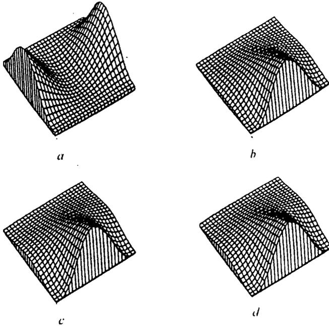
FIG. 2. The form of flexural vibrations of the panel depending on the number of approximation terms: 2a - one term ( $M = 1$ ); 2b - two terms ( $M = 2$ ); 2c - three terms ( $M = 3$ ); 2d - four terms ( $M = 4$ ).
