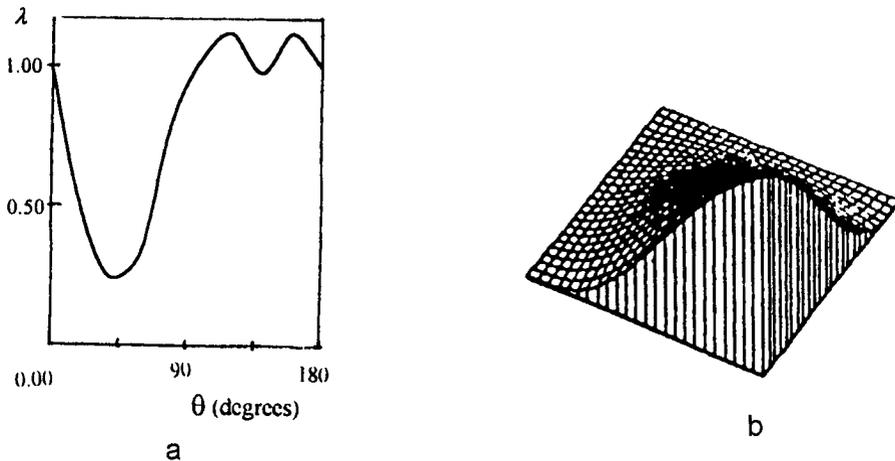
FIG. 3. Dependence of the frequency characteristic on angle  $\theta$ : 3a - first natural frequency ( $\lambda = \omega^2(\theta)/\omega^2(0)$ ) as a function of  $\theta$ ; 3b - the shape of vibrations surface  $z = 0$  at  $\theta = 45^\circ$ .
