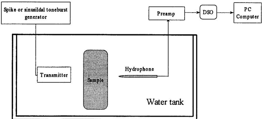
FIG. 1. Experimental setup for the ultrasonic immersion technique.
