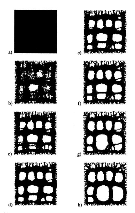
FIG. 2. Adaptation process for variable loading. a) initial state, b) -d) uniform compression in vertical and uniform tension in horizontal directions, e) -h) uniform tension in vertical and horizontal directions.
