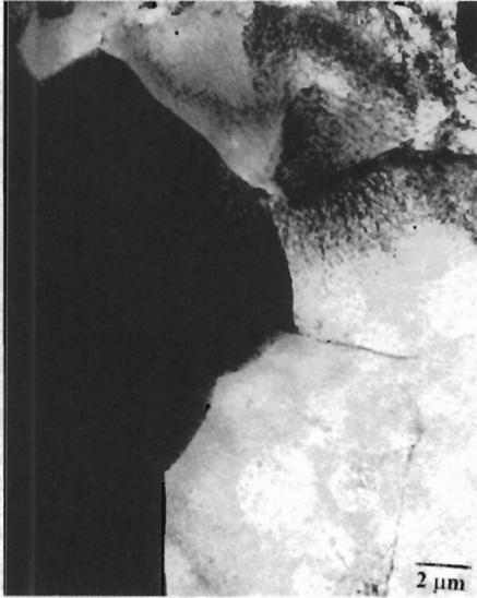
FIG. 2. Dark field TEM micrograph showing the microstructure of the Al-2.6wt.% Li-0.09wt.% Zr alloy in the overaged condition, artificially aged at 185 °C for 225 hours.
