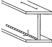
11)                       | (11) Zones of continuous longitudinal fillet or bilateral butt welds done automatically with interruptions during welding.<br>(12) Continuous longitudinal fillet or butt welds done manually. Zone of unilateral continuous longitudinal welds (especially in box girders).                                     |
