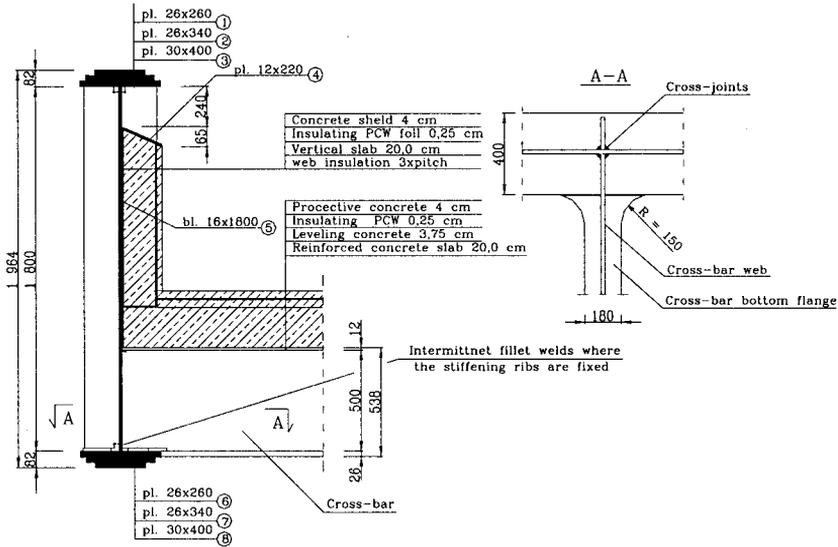
FIG. 5. Cross-section of the bridge.
