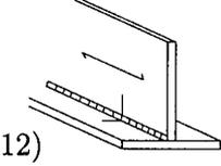
12)                       | Very good fit between wedge and flange and uniform thorough penetration without skips are required in order to obtain appropriate crack resistance on opposite side of weld.                                                                                                                                     |
