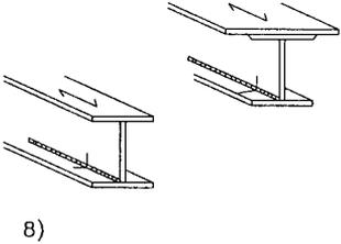
8)                    | Welded sheets and box girders –<br>– continuous longitudinal welds<br>(8) Zones of continuous longitudinal fillet welds and/or<br>(9) bilateral butt welds done automatically without interruptions.<br>(10) Zones of continuous unilateral butt welds executed automatically with backing without interruptions |
