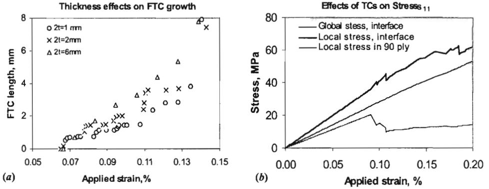
FIG. 10. Simulated transverse crack growth with the influence of the laminate thickness, (a) thickness effects on FTC growth, (b) effects of transverse cracks on  $s_{11}$ ,  $2t = 1$  mm.
