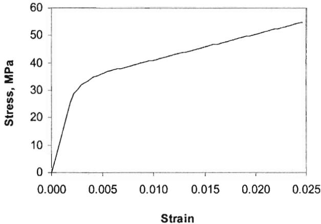
FIG. 1. The input stress-strain of the transverse layers.
