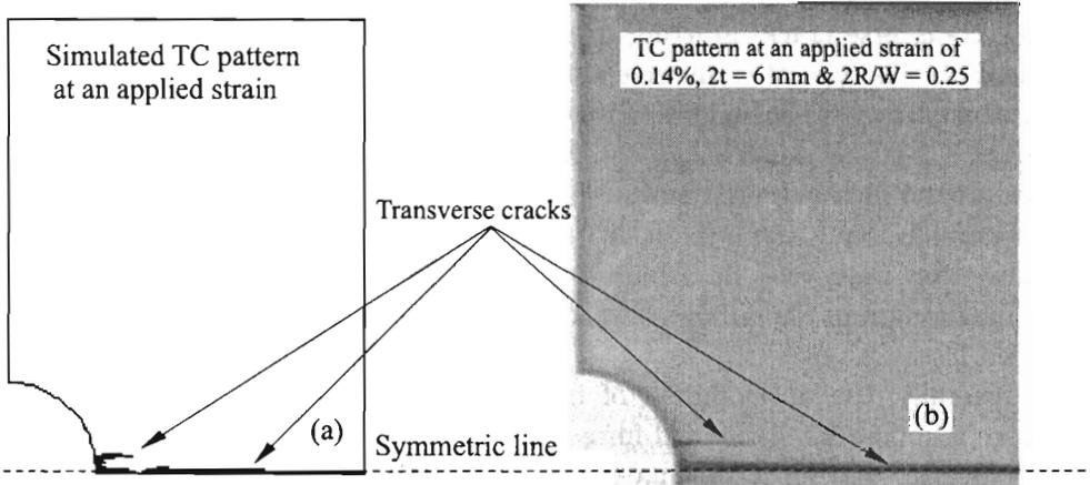
FIG. 14. Similarity of the simulated transverse cracking and the experimental observation: (a). simulated cracking pattern at  $\epsilon_{app} = 0.13\%$ , (b). observed cracking pattern at  $\epsilon_{app} = 0.14\%$ .
