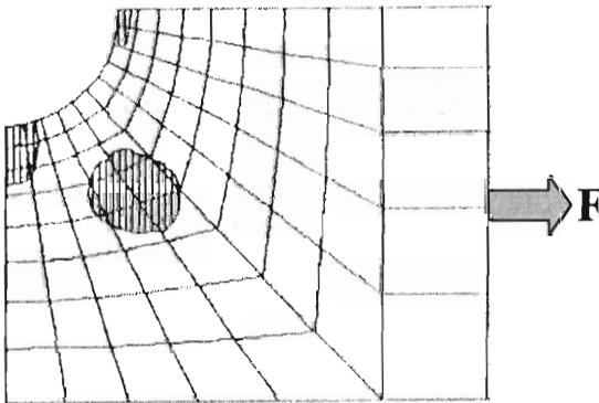
FIG. 7. Predicted damage pattern in 90° ply of AS4/3502 [0/90/ ± 45]<sub>s</sub> laminate at 276 MPa, T<sub>AN</sub> [11].
