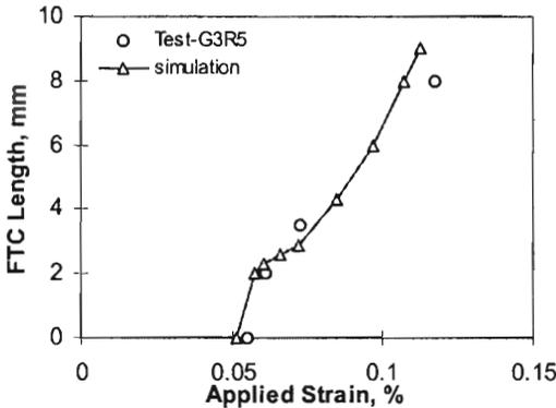
FIG. 15. Comparison of a transverse crack growth between simulation and test.
