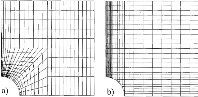
FIG. 4. Mesh orientation dependence of simulated transverse cracks: (a) unoptimized mesh, (b) optimised mesh. Simulations for a 2 mm laminate, at an applied strain 0.0014 and viewed from the symmetric surface. The darker areas represent the damaged parts in the transverse layers
