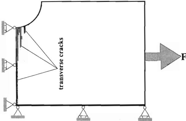
FIG. 6. Simulated transverse matrix failure pattern viewed from the 90° side at about 40 MPa.
