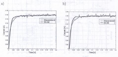
FIG. 15. Coil current flow due to step input voltage; (amplitude 1 V): a) damper filled with fluid MRF-132LD, b) damper filled with fluid MRF-336AG.
