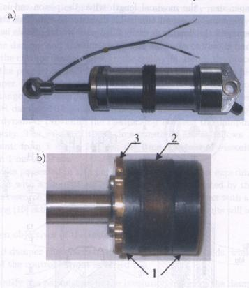
FIG. 2. a) MRF damper – general view, b) piston view: 1 - pole pieces, 2 - coil, 3 - connecting plate.
