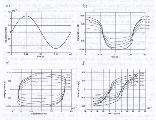
FIG. 7. Measured characteristics of the MRF damper filled with MRF-132LD, current range (0.0, 0.2) A: a) kinematic excitation vs. time, b) damping force vs. time, c) force-displacement curve, d) force-velocity curve.
