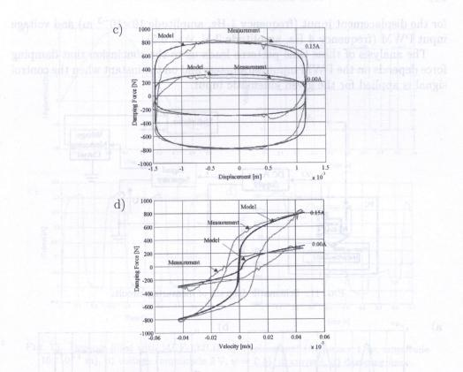
FIG. 6. Characteristics of the MRF damper filled with MRF-132LD obtained experimentally and derived from the involution model (applied current 0.0 A and 0.15 A, frequency 5 Hz): a) kinematic excitation vs. time, b) damping force vs. time, c) force-displacement curve, d) force-velocity curve.
