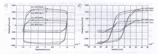
FIG. 6. Measured characteristics of the damper filled with MRF-132LD and MRF-336AG, current range (0.0, 1.4) A: a) kinematic excitation vs. time, b) damping force vs. time, c) force-displacement curve, d) force-velocity curve.
