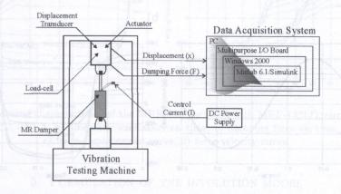
FIG. 5. Experimental setup for MR damper testing.
