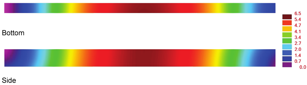
FIG. 10. Deflection map of the girder for t_w = 56 mm.
