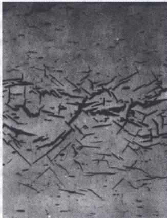
FIG. 27. Internal cleavage (penny shape) microcracks caused by shock loading in the polished cross section of an Armco iron specimen (After CURRAN, SEAMAN and SHOCKEY [19]).
