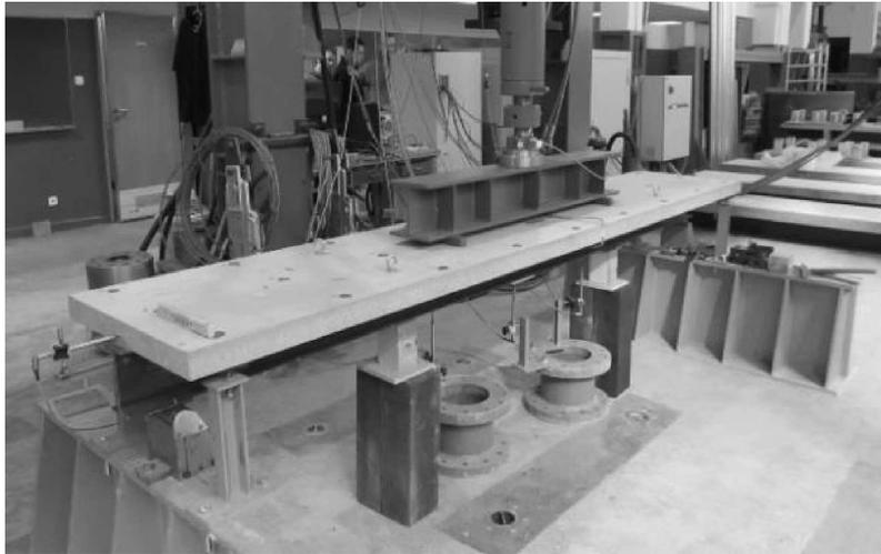
FIG. 4. Composite beam on the test stand-static load.
