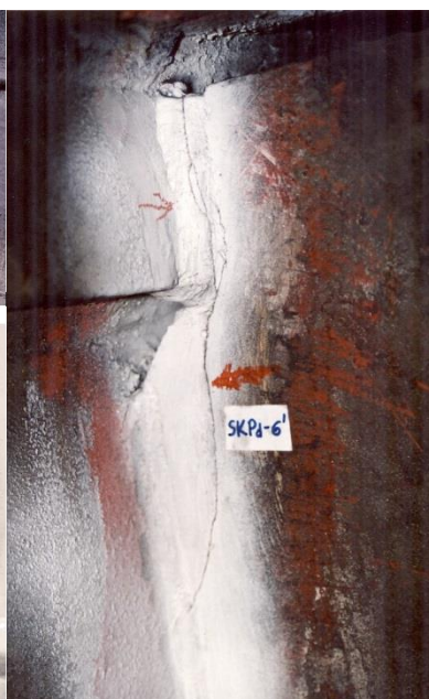
Fig. 2. Schematic presentation of the Koepe pulley with 'U' diaphragms: 1 – mantle, 2 – disk, 3 – hub, 4 – circumferential ring, 5 - diaphragm – a; fatigue cracks within a side disks zone: b – circumferential and radial cracks, c – crack in the zone joining the diaphragm 'U' with the side disk and hub [1]
