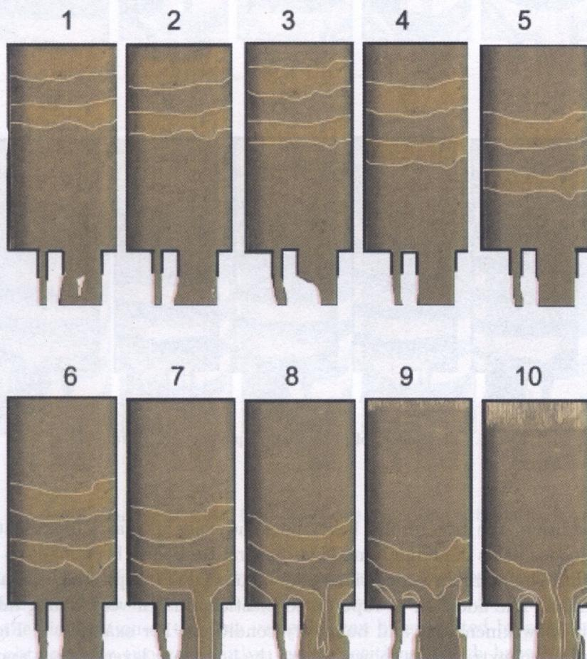
FIG. 3. The images of plastic flow – two colours of clay.
