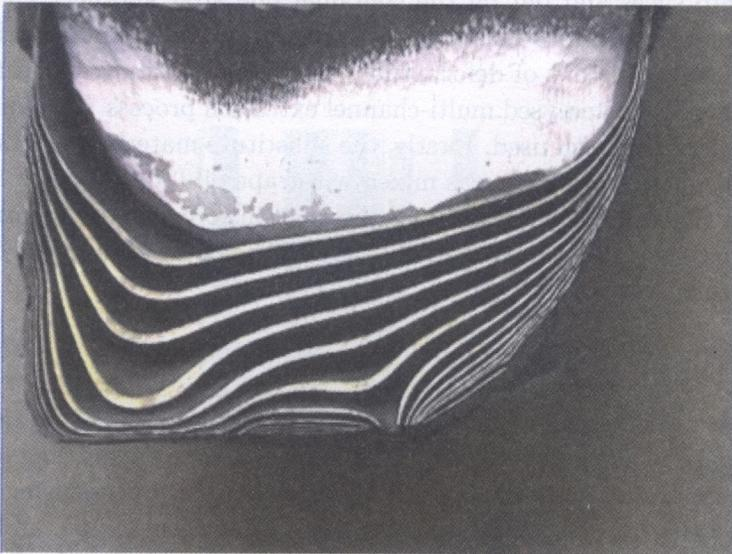
FIG. 2. Deformed layers of aluminium alloy (dual - channel extrusion).
