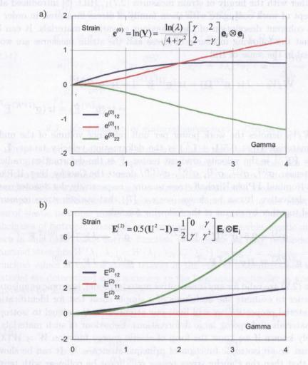
FIG. 4. Spatial (rotated) Hencky  $\underline{\mathbf{e}}^{(0)} = \underline{\mathbf{R}} \underline{\mathbf{E}}^{(0)} \underline{\mathbf{R}}^T = \ln(\underline{\mathbf{V}})$  and Green Lagrange  $\underline{\mathbf{E}}^{(2)} = 0.5 (\underline{\mathbf{U}}^2 - \underline{\mathbf{I}})$  strain tensors components, expressed in a fixed laboratory coordinate frame, as functions of the deformation parameter  $\gamma$ .
