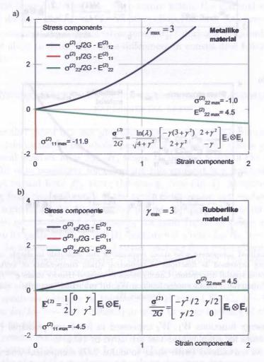
FIG. 5. Normalized component-wise stress response of two materials submitted to simple shear deformation loading expressed as functions of the respective strain components of workconjugate strain measure in material description, II Piola–Kirchoff stress  $\leftrightarrow$  Green Lagrange strain  $\underline{\sigma}^{(2)}/2G \leftrightarrow \underline{E}^{(2)}$ , a) "metallike" material – elastic energy function  $\hat{W}_2$ , b) "rubberlike" material – elastic energy function  $\hat{W}_1$ .
