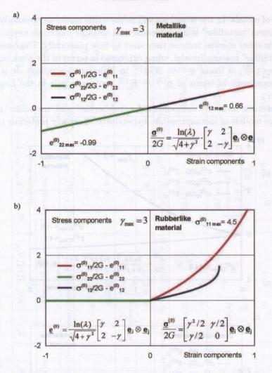
FIG. 6. Normalized component-wise stress response of two materials to simple shear deformation loading expressed as functions of respective strain components of work-conjugate strain measure in spatial description, Cauchy stress  $\leftrightarrow$  rotated Hencky strain  $\underline{\sigma}^{(0)}/2G \leftrightarrow \underline{\mathbf{e}}^{(0)}$ , a) "metallike" material – elastic energy function  $\hat{W}_2$ , b) "rubberlike" material – elastic energy function  $\hat{W}_1$ .
