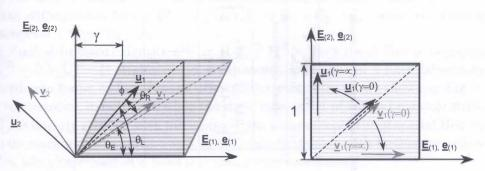
FIG. 3. Homogeneous simple shear. Location of Lagrangian  $\underline{\mathbf{u}}_1$  and Eulerian  $\underline{\mathbf{v}}_1$  eigenvectors with increasing deformation parameter  $\gamma$ . On the right, initial ( $\gamma = 0$ ) and final ( $\gamma = \infty$ ) positions of vectors  $\underline{\mathbf{u}}_i$ ,  $\underline{\mathbf{v}}_{\alpha}$  are shown.
