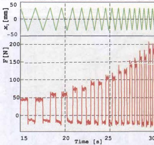
FIG. 2. Displacement and damping force in the function of time in the part of the experimental program.
