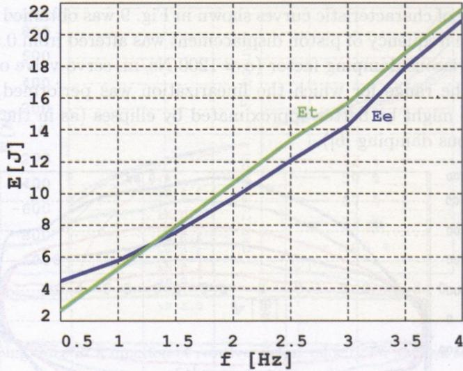
FIG. 11. The amount of energy dispersed in one cycle as a function of frequency, 50% servo-valve opening.
