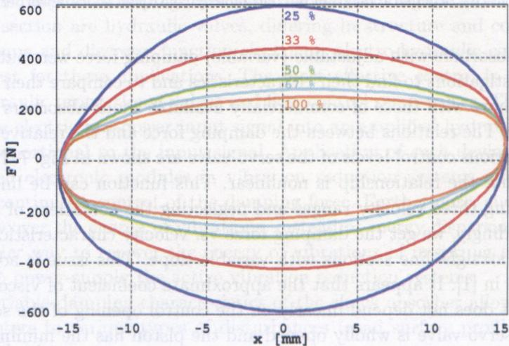
FIG. 8. Damping force as a function of piston displacement for various control openings of the servo-valve, vibrations frequency 3 Hz.
