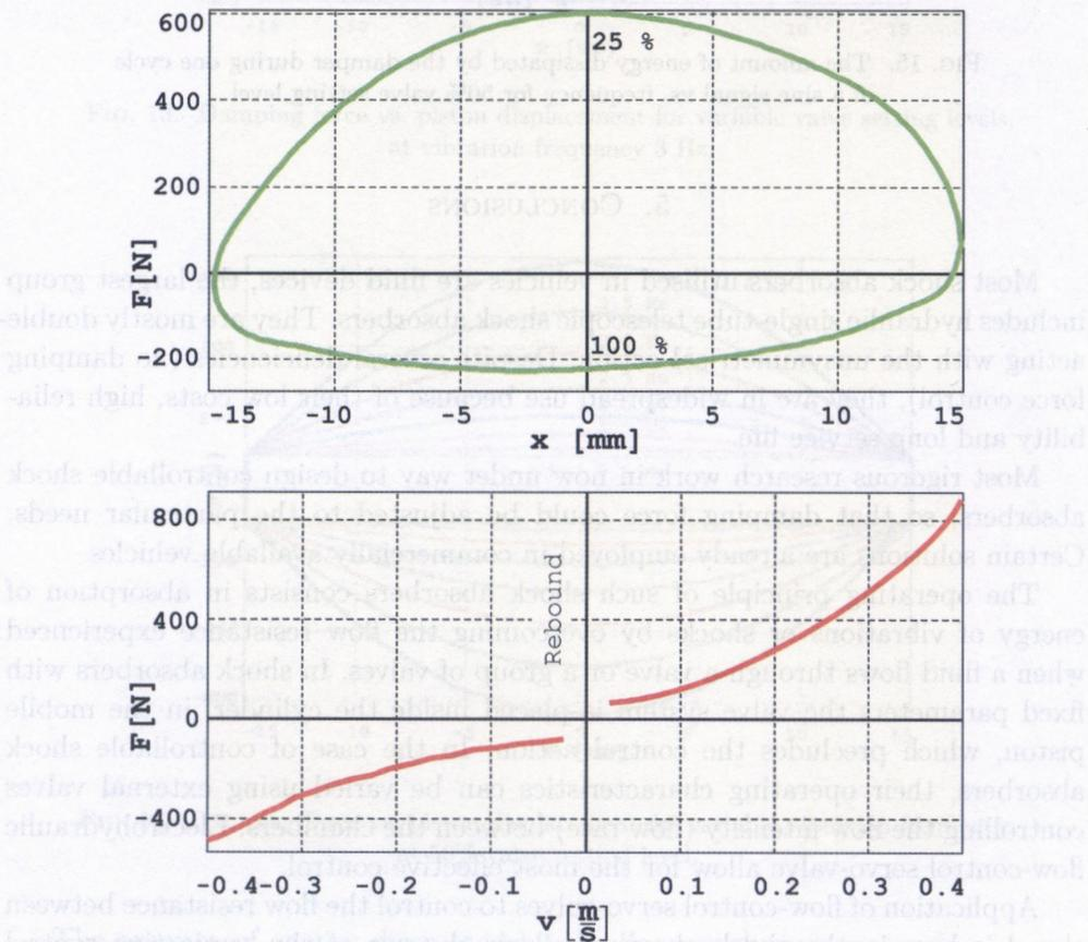
FIG. 16. Shaping the characteristics of a controllable servo-valve.
