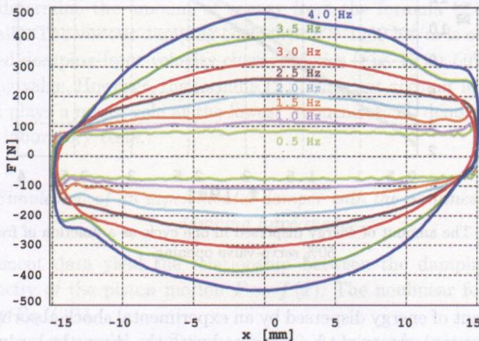
FIG. 9. Damping force as a function of piston displacement for various vibration frequencies, 50% servo-valve opening.
