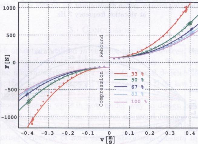
FIG. 12. Comparison of experimental characteristics and those derived from the nonlinear model.
