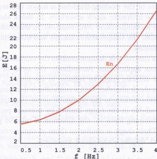
FIG. 15. The amount of energy dissipated by the damper during one cycle of a sine signal vs. frequency for 50% valve setting level.
