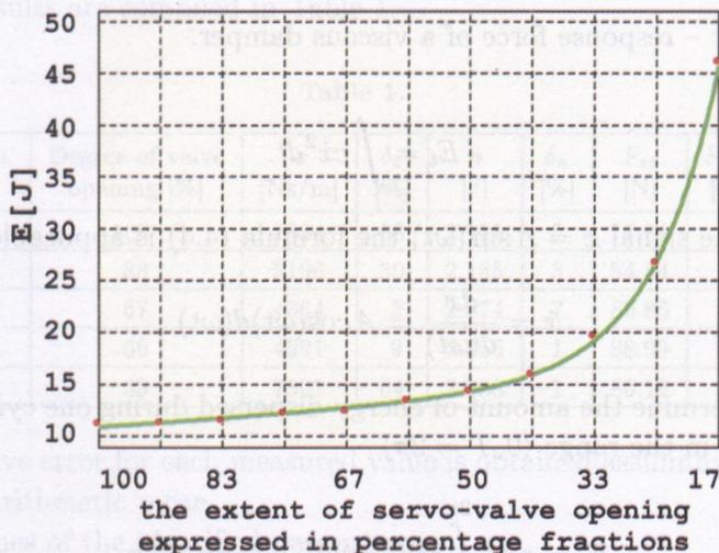
FIG. 10. The amount of energy dispersed in one cycle depending on the servo-valve opening.
