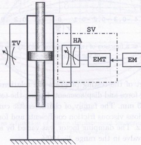
FIG. 6. Schematic diagram of continuously controlled shock absorber.
