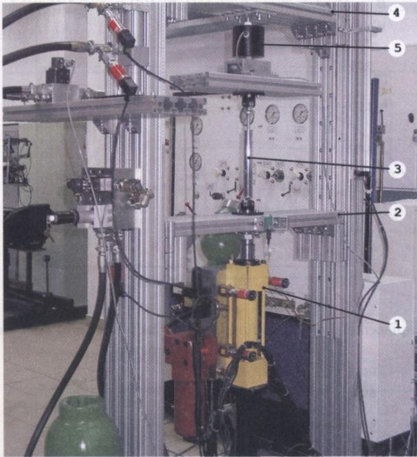
FIG. 1. Experimental stand with a commercially available shock absorber mounted in between the platforms.
