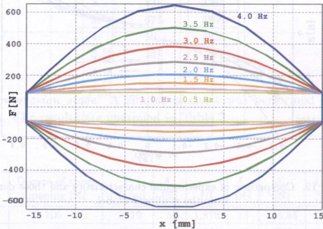
FIG. 14. Damping force vs. piston displacement for variable vibration frequency, at 50% valve setting level.
