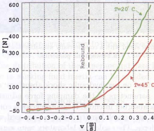
FIG. 3. Comparison of damping characteristics depending on the piston velocity for two oil temperatures.
