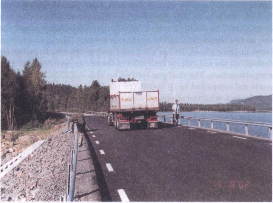
FIG. 4. Rear view of ballasting truck on bridge during tests (symmetric load scheme II).
