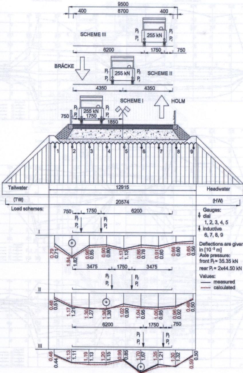
FIG. 6. Graphs of maximum vertical displacements in transverse direction of the span for three test load schemes.
