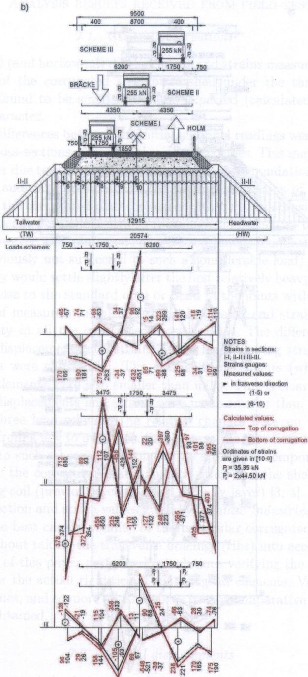
FIG. 9b. Graphs of maximum strains in selected points (gauges no. 1-20 in longitudinal direction) of steel shell structure in cross-sections of the span: b) II-II.
