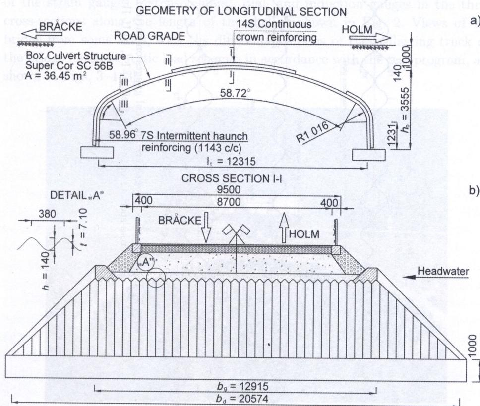
FIG. 1. Road bridge in Gimån, Sweden, made form Super Cor SC-56B corrugated plates:
