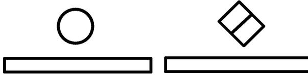
FIG. 1. Impact cases: a) sphere, b) cube corner.
