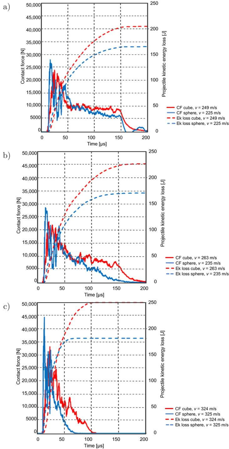
FIG. 10. Contact forces for impacts: a) below, b) above, and c) 325 m/s.
