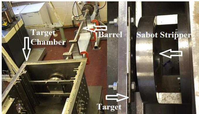
FIG. 2. Experimental setup: overview.
