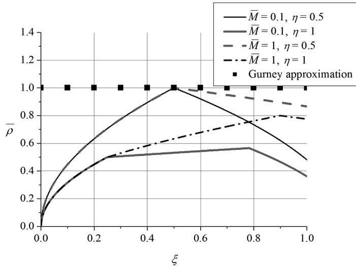
FIG. 5. Variation of the relative density,  $\bar{\rho}$ , of the DPs versus Lagrangian coordinate,  $\xi$ , for selected values of  $\eta$  and  $\bar{M}$ .
