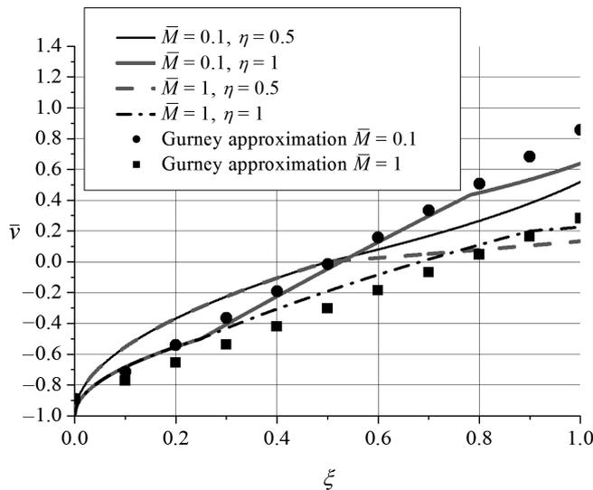
FIG. 4. Variations of the relative velocity,  $\bar{v}$ , of the DPs versus Lagrangian coordinate,  $\xi$ , for selected values of  $\eta$  and  $\bar{M}$  (on the background linear Gurney approximation).
