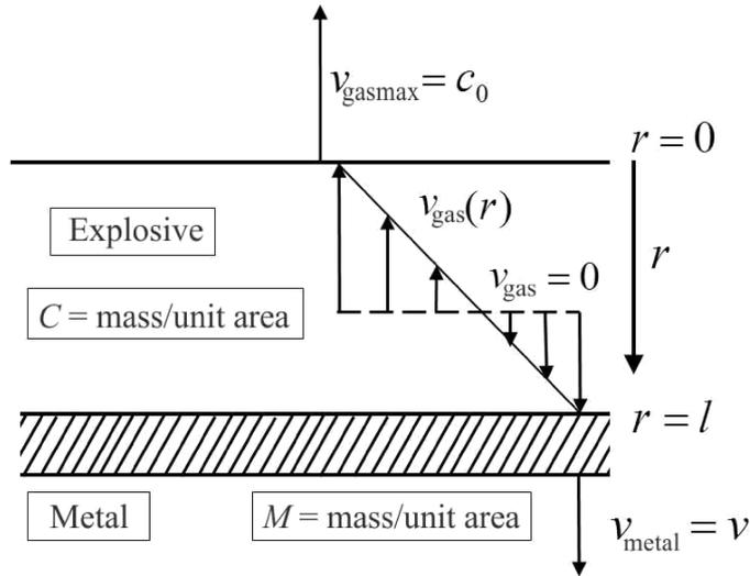
FIG. 2. The linear profile of DPs velocity versus Lagrangian coordinate,  $r$ , for an OFS.
