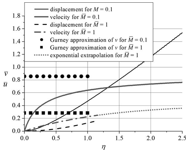
FIG. 6. Variation of the relative displacement and velocity of metal plate versus relative time  $\eta$ , for selected values of  $\bar{M}$ .
