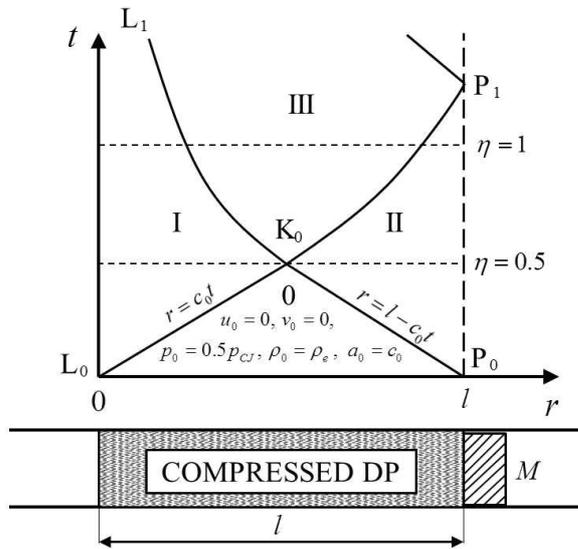
FIG. 3. Part of the network of limiting characteristics in the space between piston and free surface.
