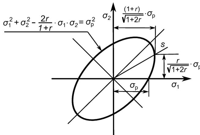
FIG. 1. Stress condition arising at the H-M-H yield ellipsis at the onset of instability.
