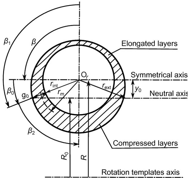
FIG. 11. Schematic picture of cross-section of the elbow and its characteristic parameters.
