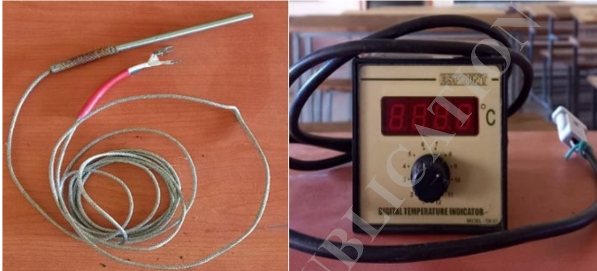
Figure 5. Thermocouple and temperature indicator.
