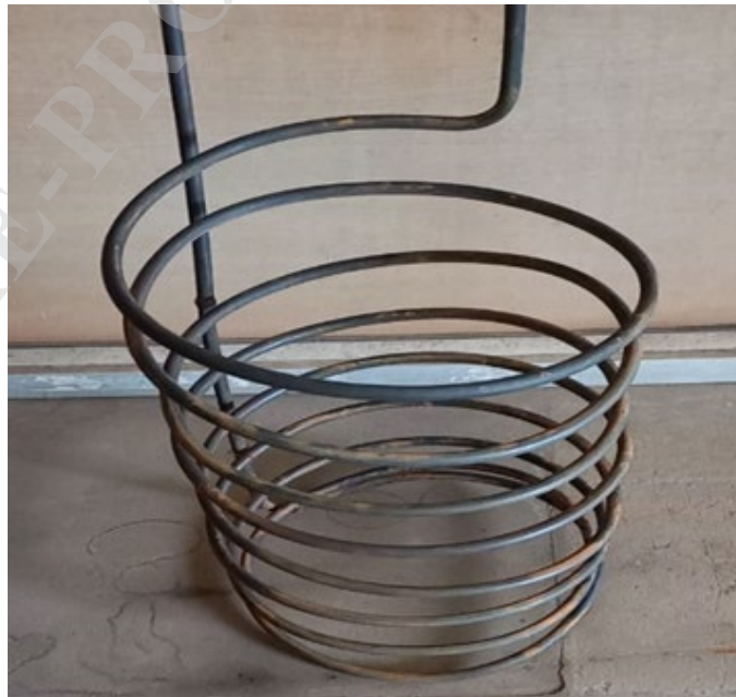
Figure 4. Fabricated copper coil heat exchanger.
