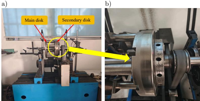
FIG. 1. Imbalance detection of the impeller body using a dynamic balancing machine (a), angle indicator on the dynamic balancing machine (b).
