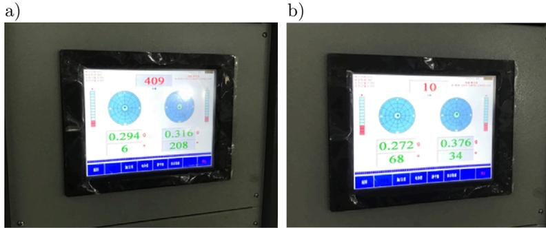
FIG. 3. Residual unbalance of the impeller body during rotation after achieving balance (a), and at rest after achieving balance (b).
