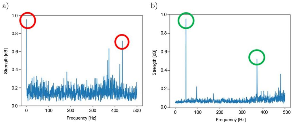
FIG. 6. Frequency domain analysis: a) frequency-domain diagram of the vibration signal at position 1 before optimization, b) frequency-domain diagram of the vibration signal at position 2 before optimization.
