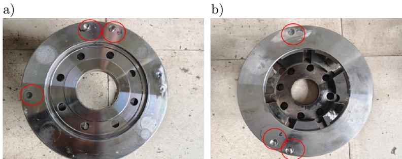
FIG. 2. Evaluation of the primary disk of the impeller body following dynamic balancing (a), examination of the auxiliary disk of the impeller body after dynamic balancing (b).
