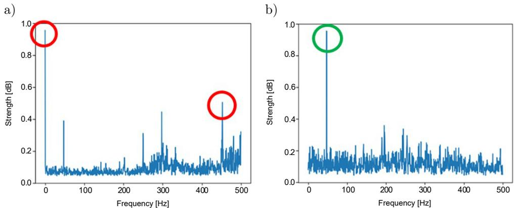
FIG. 7. Frequency-domain analysis: a) frequency-domain diagram of the vibration signal at position 1 after optimization, b) frequency-domain diagram of the vibration signal at position 2 after optimization.
