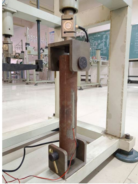
Fig. 3 Suspension rod loading device.
