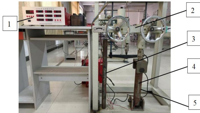
Fig. 4 Schematic diagram of the tensile force application platform: 1. strain indicator, 2. mechanical loading platform, 3. temperature compensator, 4. strain gauge, 5. suspension rod.
