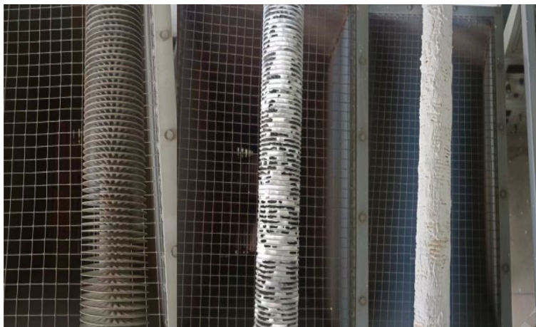
Fig. 6. Schematic diagram of ash deposition distribution.
