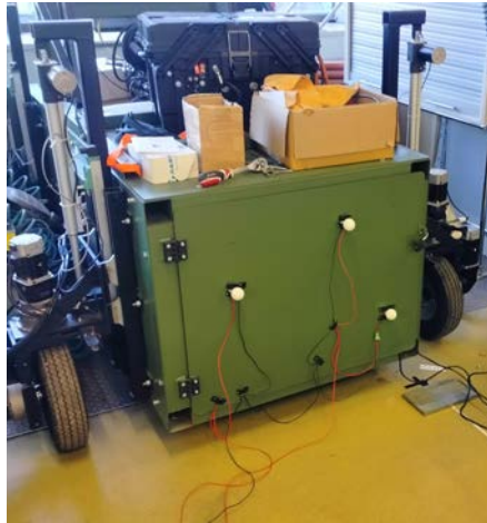
FIG. 9. The measuring station – light markers installed on a vehicle capable of uniform up-and-down movement.
