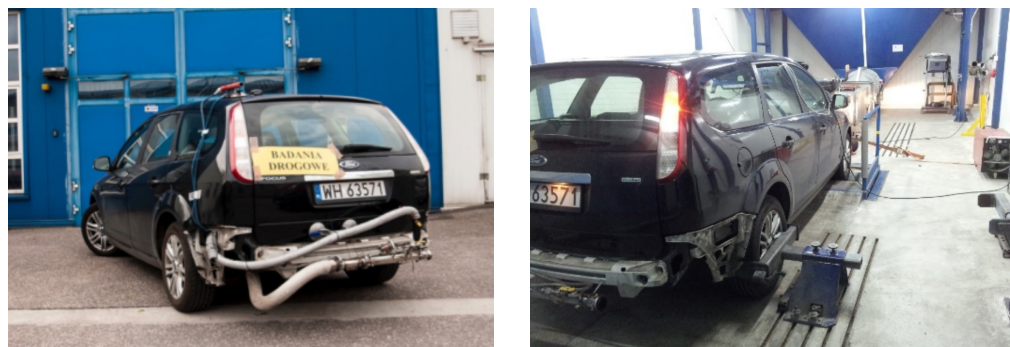
FIG. 1. Test vehicle equipped with Semtech DS testing equipment.
