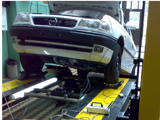
FIG. 3. Measurement of normal forces under the front axle wheels after lifting the front axle about 0.5 m.
