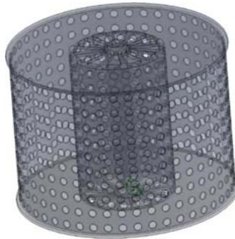
FIG. 15. Model of the centrifugal extractor drum.
