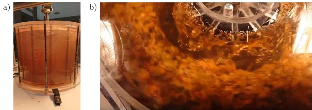
FIG. 19. Test setup for studying liquid flow in the extractor drum: a) view of the setup, b) liquid flow in the drum filled with material.
