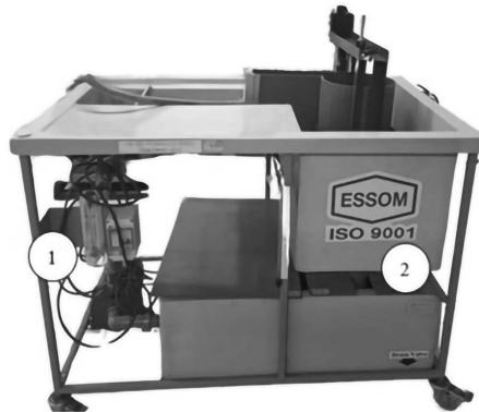
FIG. 4. Experimental setup of the GWVT and hydraulic bench.
