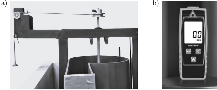
FIG. 5. Devices used to measure: a) brake power, and b) RPM.
