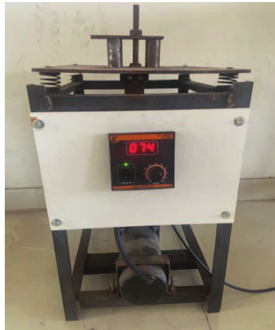
FIG. 3. Photograph of the actual test setup used for VSR.
