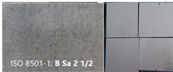
FIG. 1. Visual inspection of the material after the sandblasting process, according to ISO 8501-1 [28].
